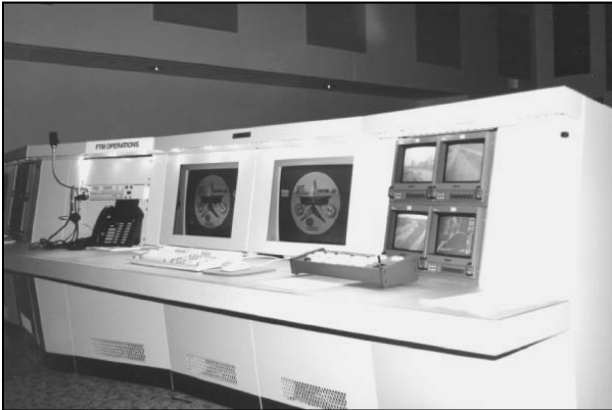
Figure 10-5. Typical Operator Workstation in the Houston TranStar Freeway Management Control Center.
