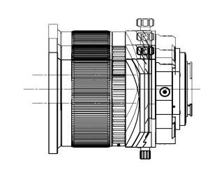
The shifting knob is black and the locking knob is gray. Use the black knob to adjust the shifting and rotate the gray knob in the L direction to hold it in place.
