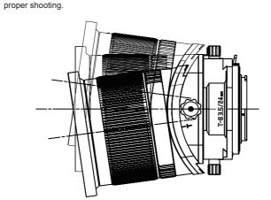
Make sure to differentiate the knob for tilting. The tilting knob is black and the locking knob is gray. Use the black knob to adjust the tilting and rotate the gray knob in the L direction to hold it in place.
