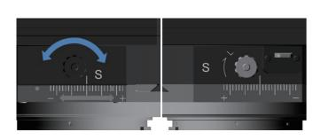
If the amount of shift is large, the lighting may be different at the top or bottom of the image, or on the left or right of the image. Therefore it is recommended to reduce the aperture value when shooting.
